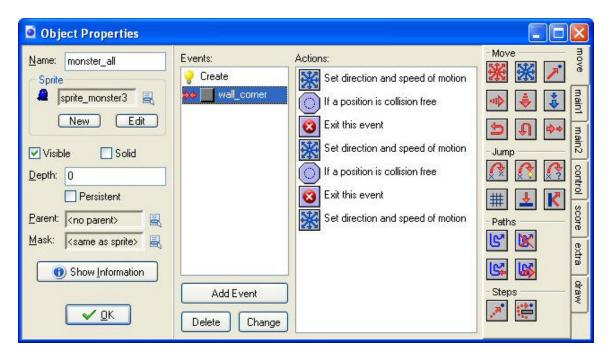
To avoid problems with monsters being slightly too small, we uncheck precise collision checking and set the bounding box to the full image.
