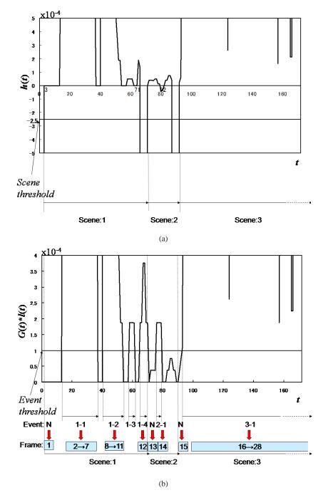
**Fig. 2** (a) Scene partition based on h(t), (b) event extraction based on G(t) \* l(t).
